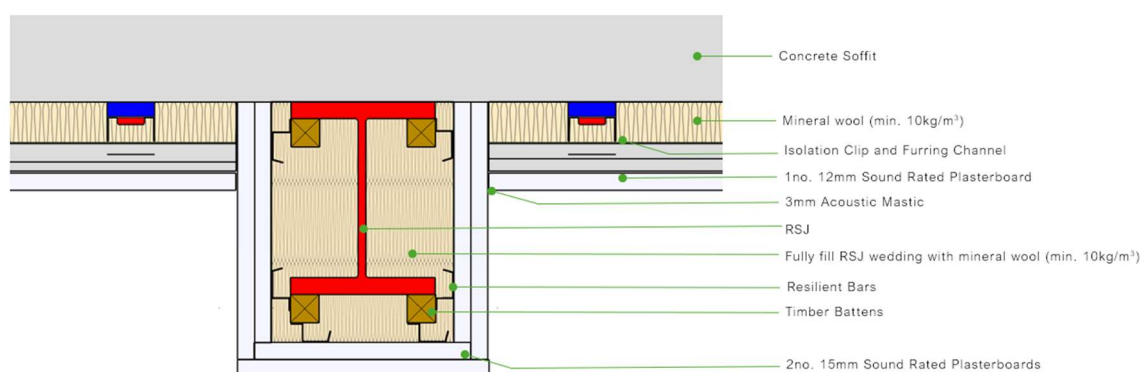
Figure 7 – RSJ Ceiling Boxing Detail – Resilient Bars
