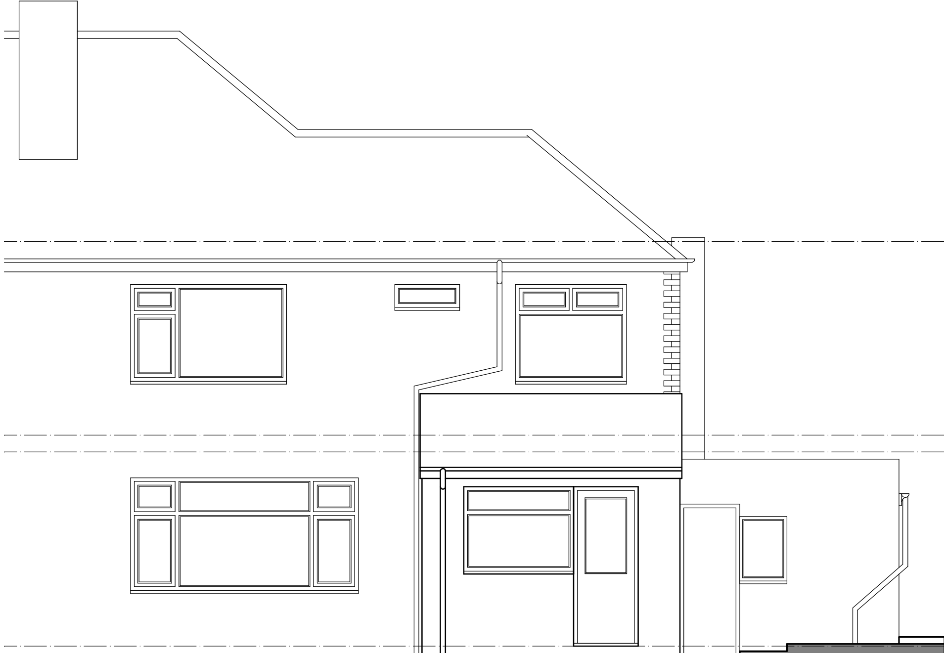
existing rear elevation
