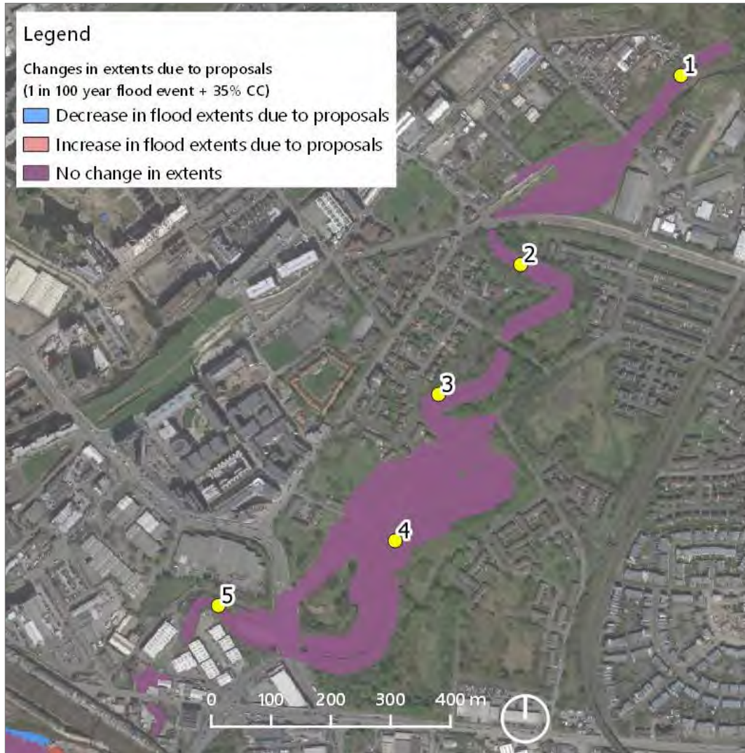
Figure 5.7 – Comparison of Mayfield 2019 model to the BHE Baseline 2019 model, flood extent changes for the DFE, upstream of site.
