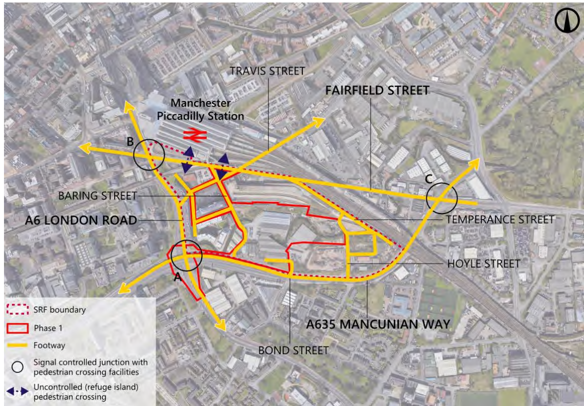
Figure 3.2 Pedestrian Infrastructure Surrounding the Site
