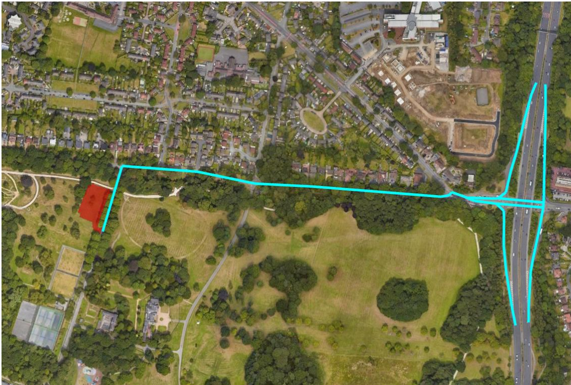
Figure 2: Construction Traffic Routeing
