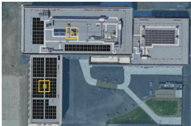
Fig.3 – Position of the proposed PV panels
