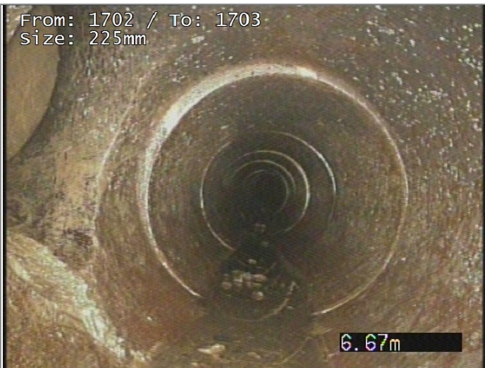
Junction, closed at 10 o'clock, diameter 100mm
