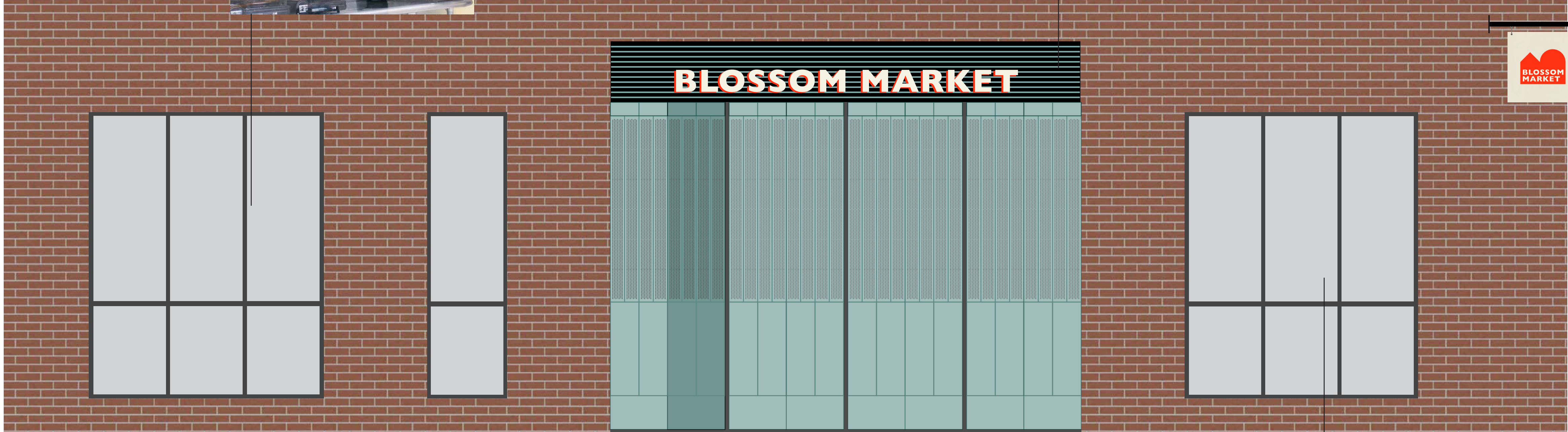
TENANT BRAND SIGNAGE WINDOW VINYL OR PAINT APPLIED DIRECTLY TO THE GLAZING WILL BE USED MINIMALLY AND TASTEFULLY TENANT WILL BE REQUIRED TO GAIN LANDLORD APPROVAL BEFORE APPLICATION VINYL SHOULD COVER NO MORE THAN 25% OF THE OVERALL GLAZING
