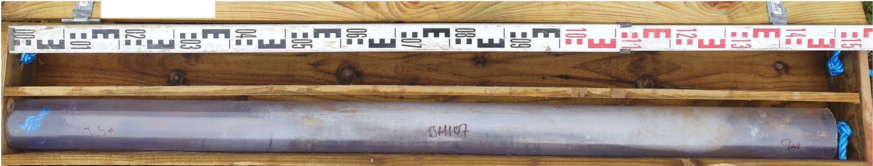
BH107 Box 1 CORE RUN 1 7.5m – 9.0M
