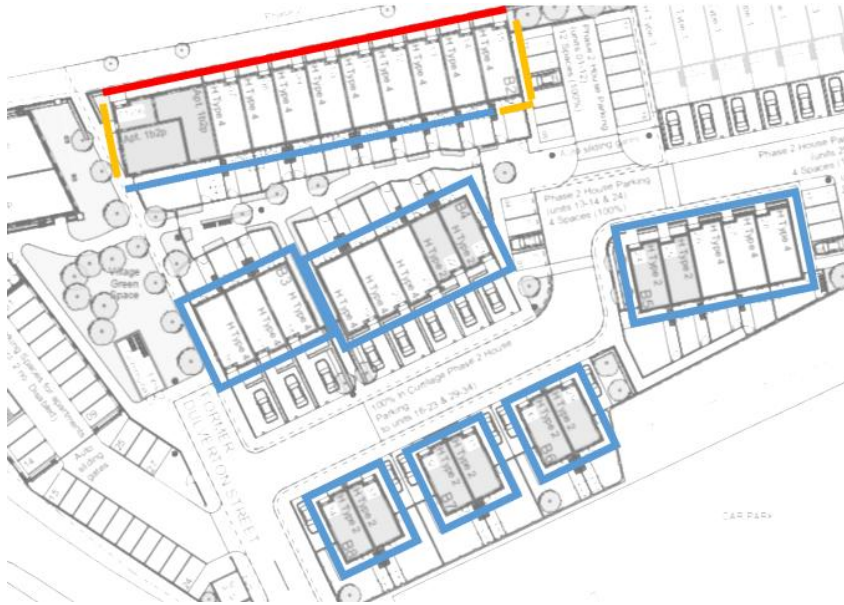
Façade acoustic specification zones (all levels)
