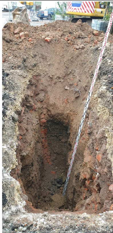
Plate No. 19: PP TPI10 concrete footing extending 1.0m and 0.5m deep, founded on sandstone
