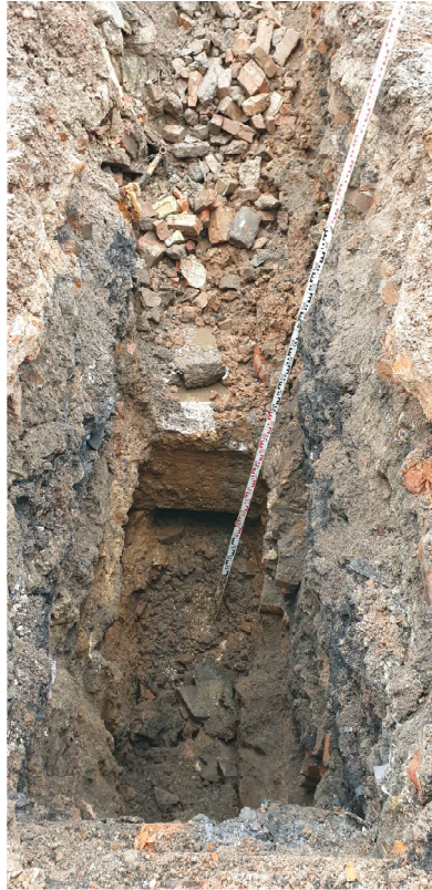
Photo No. 45: TP313 – concrete block at 2.0 -2.8m in southern pit face
