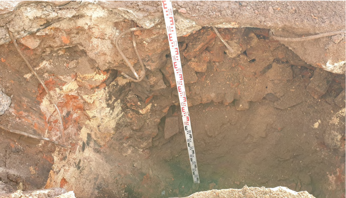
Soil sample obtained for leachate analysis in pit at depth of 1.95m
