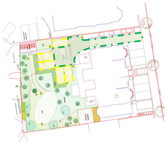
Figure 2.1 Plan view showing proposed site layout (image © simon james arq ltd)
