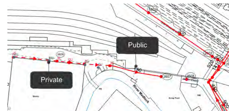
Figure 6-2 Known private site sewerage (Image courtesy of the United Utilities © United Utilities Water PLC 2017)
