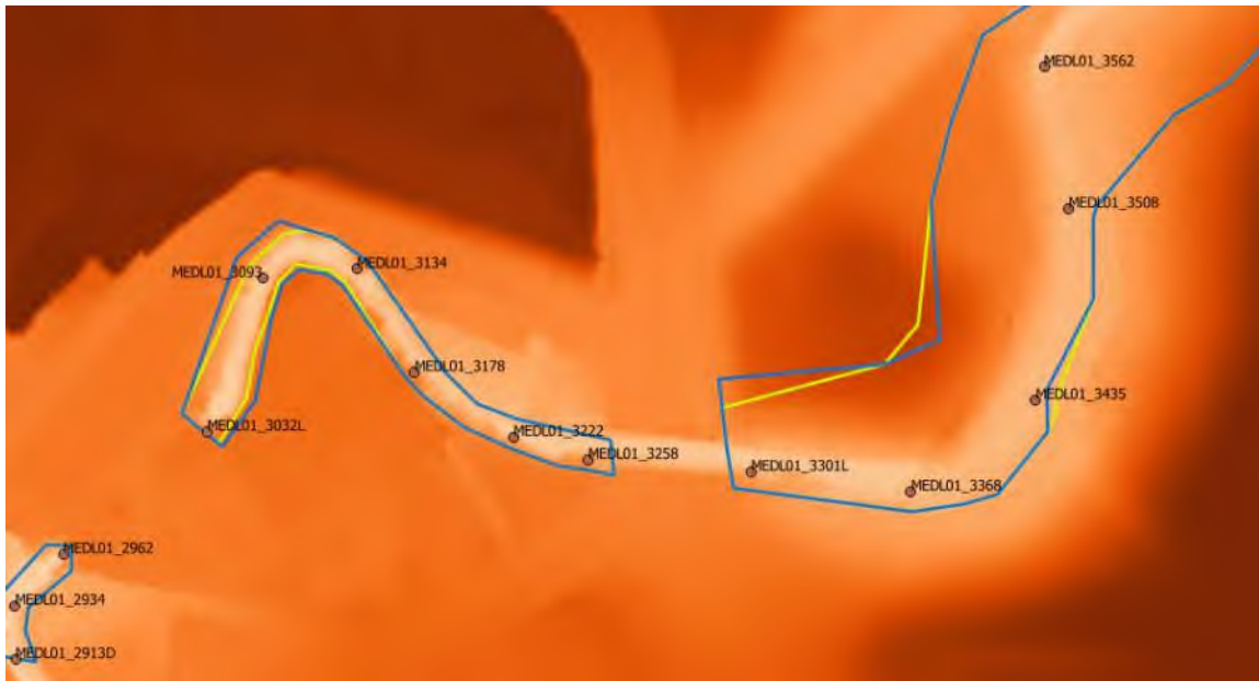
Figure 4.3 - 1D space around Pin Mill Brow area (blue – Medlock 2008 model, yellow – BHE Baseline 2019)
