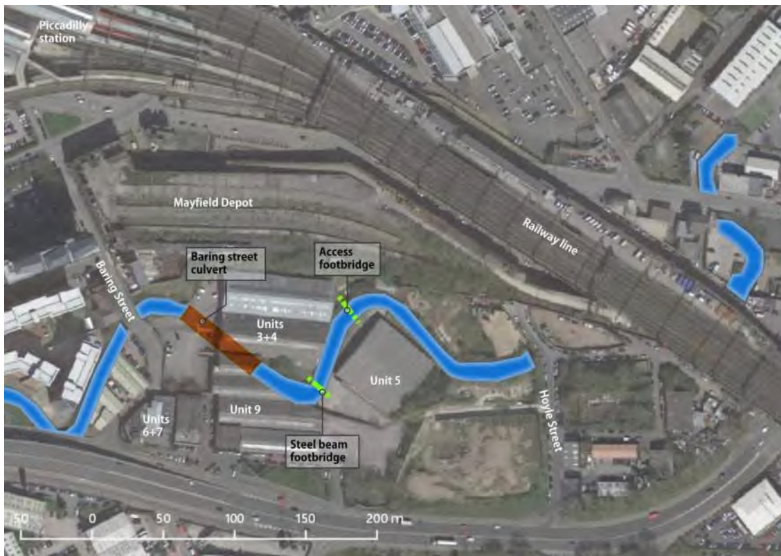
Figure 4.7 - Mayfield site - existing assets. Open watercourse shown in blue.
