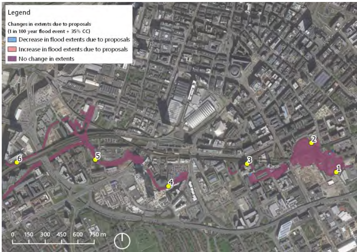
Figure 5.8 - Comparison of Mayfield 2019 model to the BHE Baseline 2019 model, flood extent changes for the DFE downstream of site.
