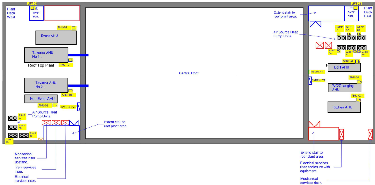
Figure 1: RIBA stage 2 roof plant layout sketch
