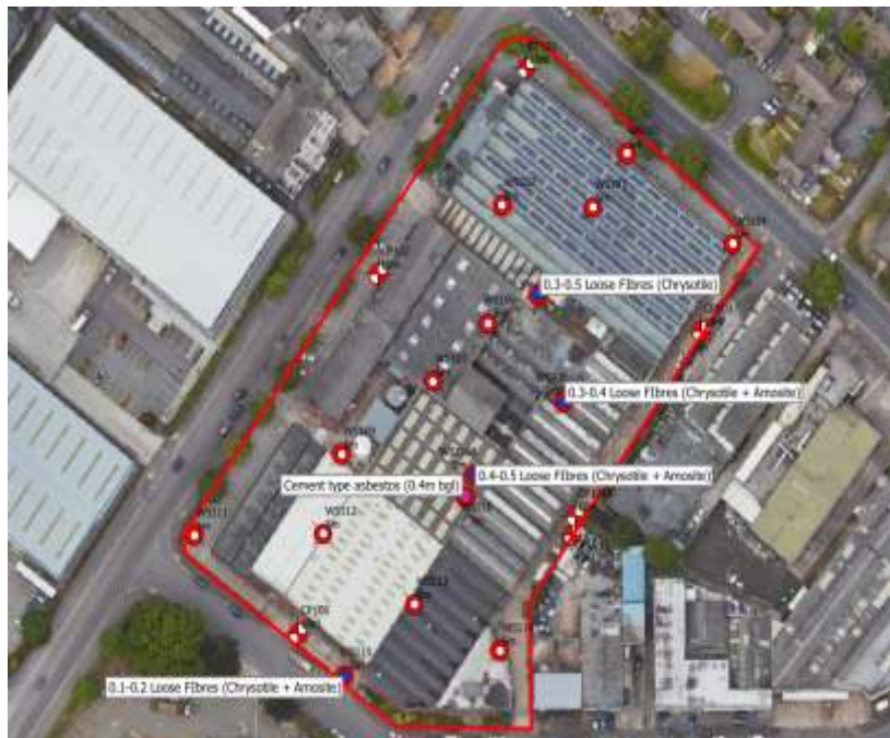
Figure 2.2: Location of laboratory confirmed cement type asbestos
