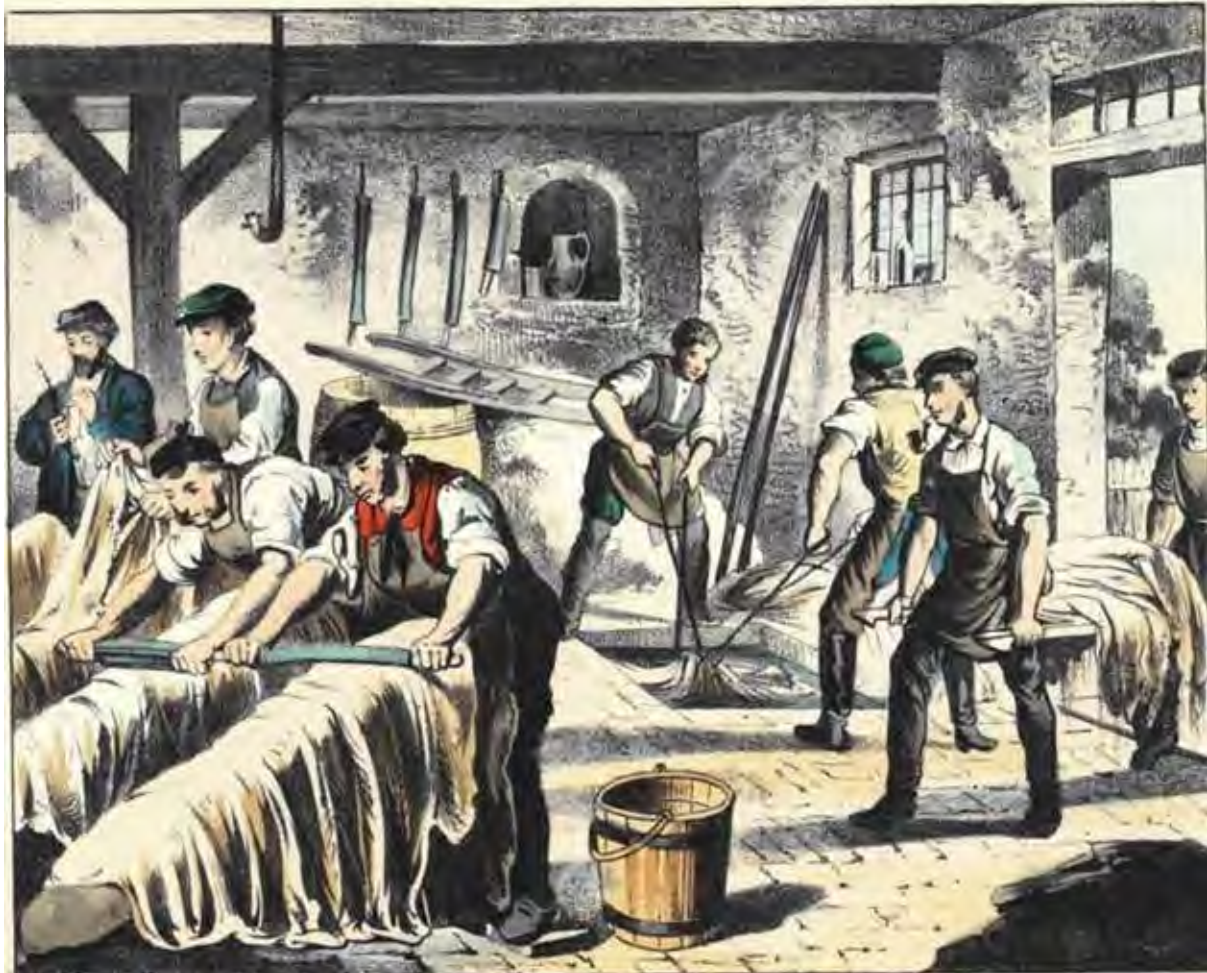
Plate 6: Image illustrating the process of scouring in a late 19 th century tannery (Courtesy of the Hagen History Centre)
