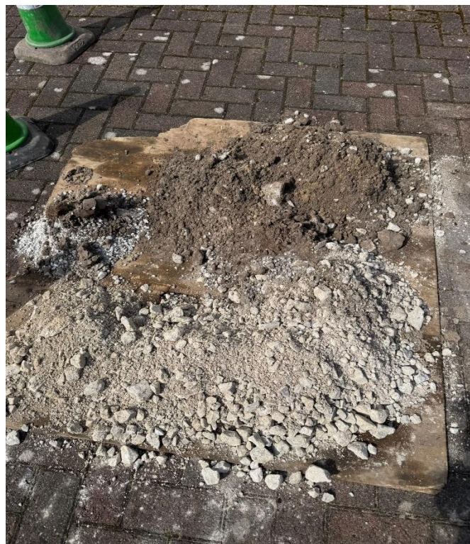
Plate 6 – WS02 GL to 1.00m bgl. Hand pit arisings
