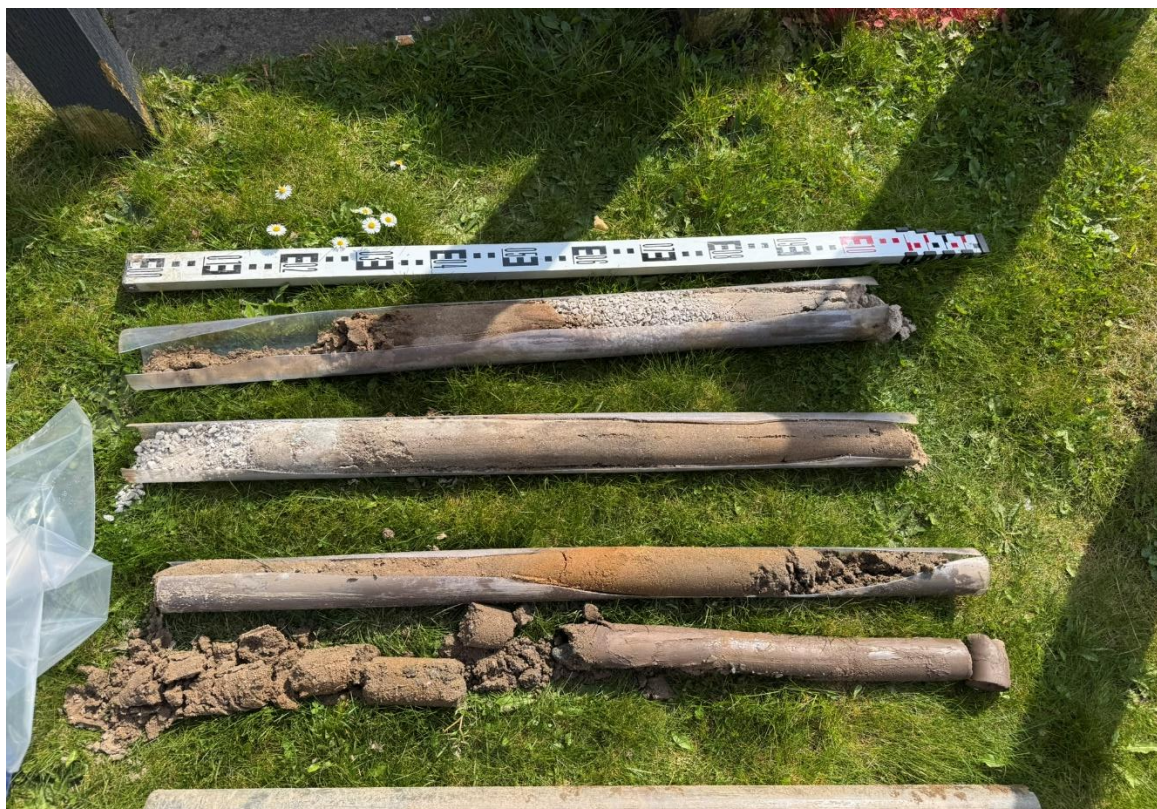
Plate 1 – Window Sampler borehole (WS01) 1.0m bgl to 5.00m below ground level (bgl)
