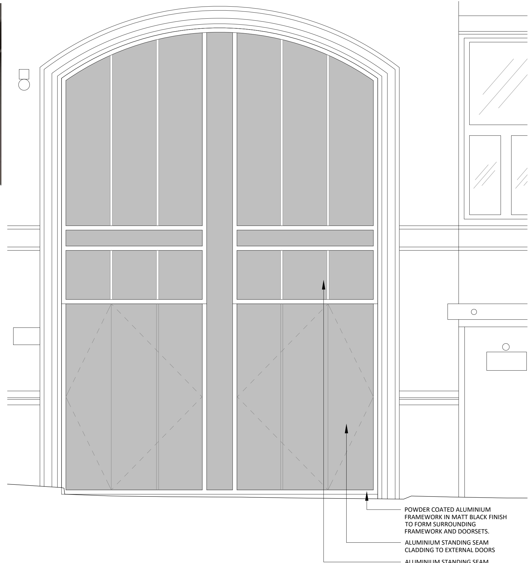
07 NEW ESCAPE DOOR ELEVATION 140 SCALE - 1:20 @ A1
