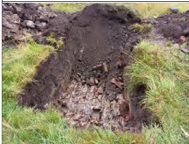
Photo 3: Showing made ground and brick wall in TP04, facing south west.
