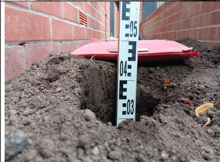
Photograph 3: Depth measurement in Pit 2.
