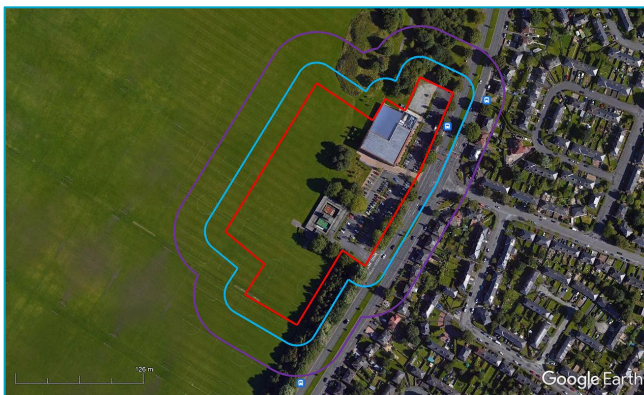
Figure 5. Earthworks boundary with 20m and 50m buffers
