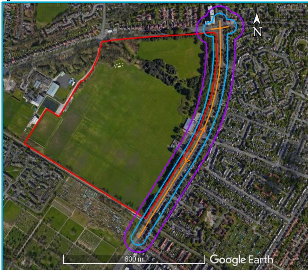
Figure 7. Trackout route with 20 m and 50 m buffers
