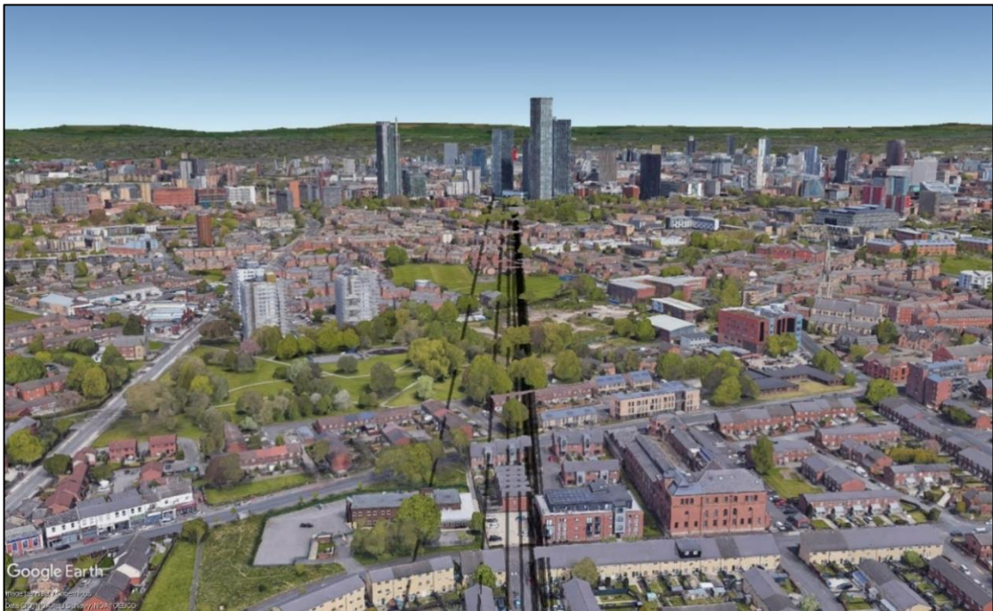
Figure 9 Intervening tall buildings blocking SSR line of sights towards proposed development
