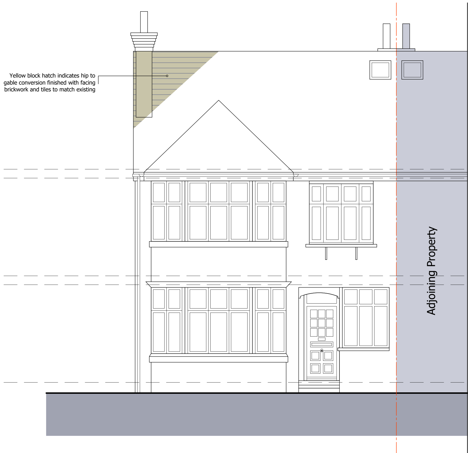
FRONT ELEVATION (North East)
