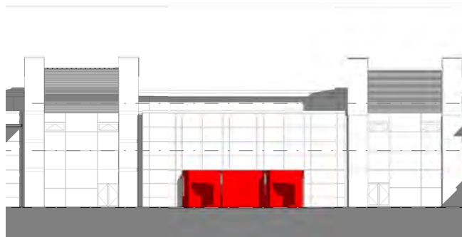
Existing Entrance Demolition
