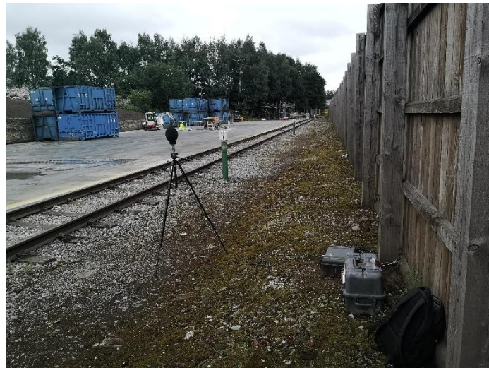
Figure 1.1 Long-term Unattended Sound Level Measurement Position – MP1
