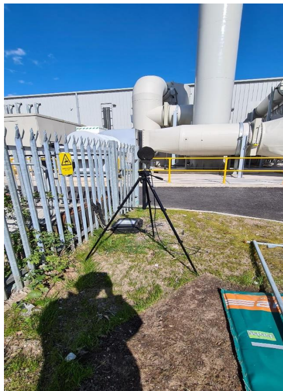
Figure 1.2 Long-term Unattended Sound Level Measurement Position – MP2
