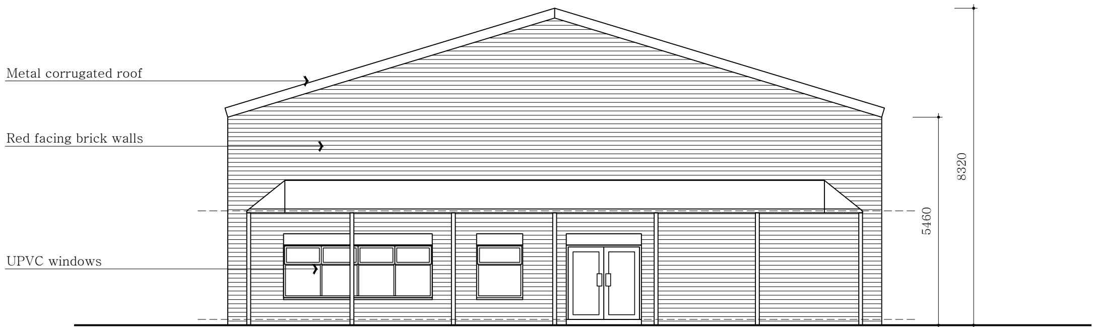
EXISTING FRONT ELEVATION (S) 1:100
