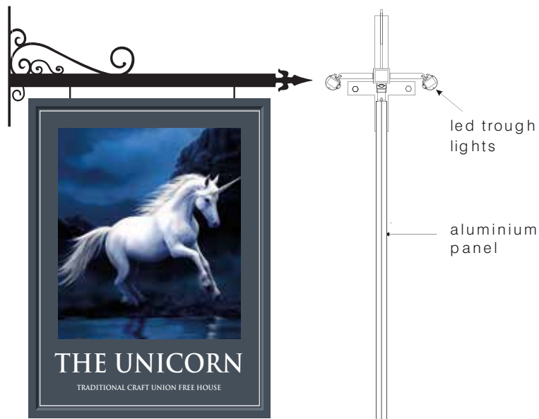
Sign A Aluminium projecting sign complete with steel gibbet Illuminated by led trough lights. Sizes 900 x 1200mm, Projection - 1140mm. G/Cl - 4790mm, D - 40mm.
