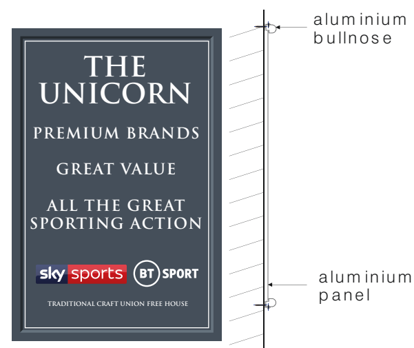
Sign C Two aluminium bullnose boards. Sizes 700 x 1100mm, G/Cl - 1490mm, D - 40mm.
