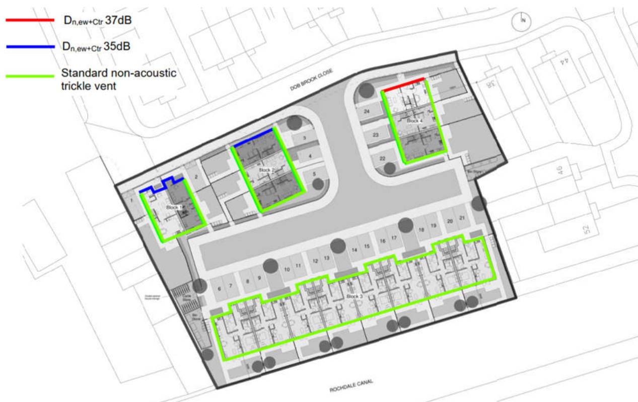
Figure 3 Ventilator performance mark-up
