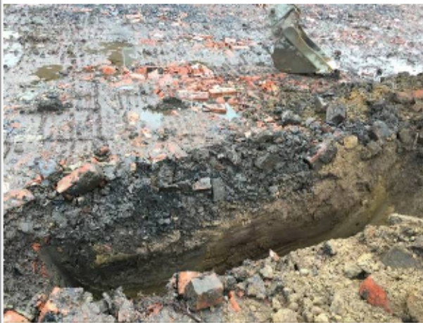
Photo 4: Trial Pit 2. East edge of pit showing layering of Made Ground over Glaciofluvial sand.
