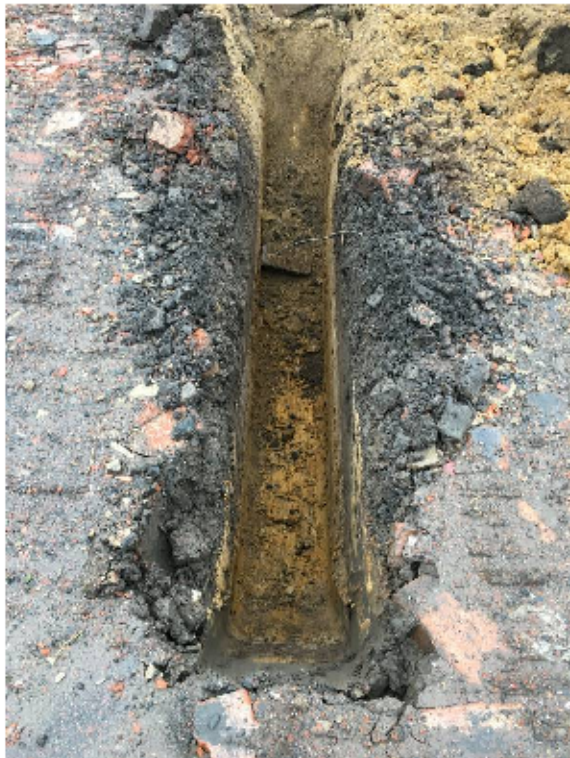
Photo 3: Trial Pit 1. Showing Made Ground over natural Glaciofluvial sand.
