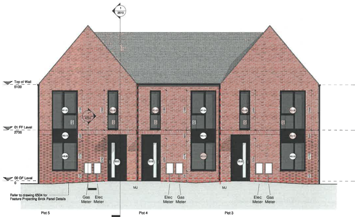
Front (East) Elevation 1 : 50
