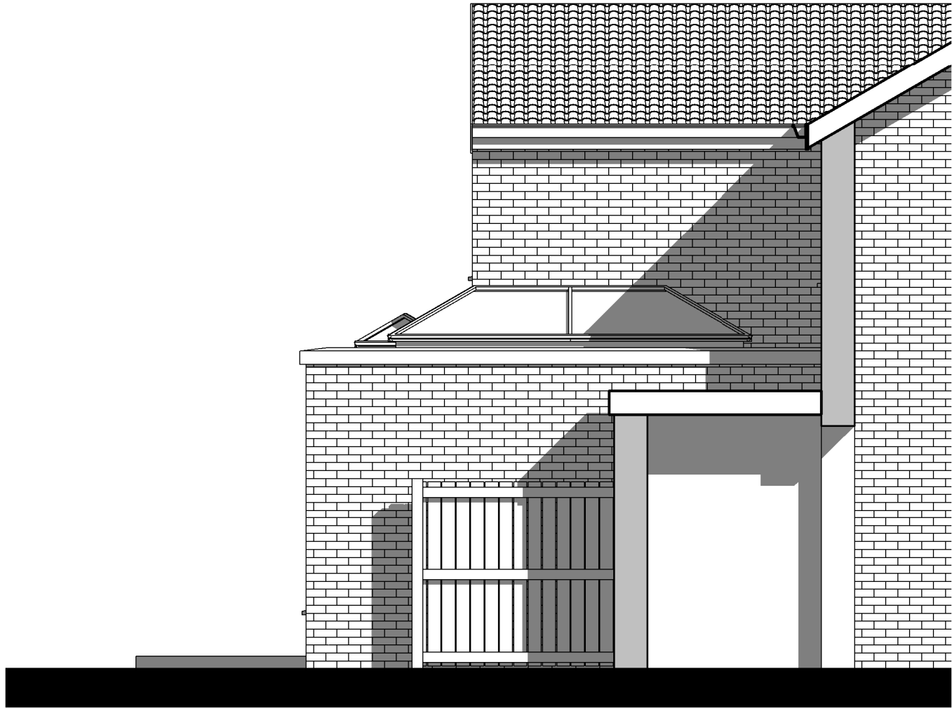
Proposed Side Elevation1 1 : 50
