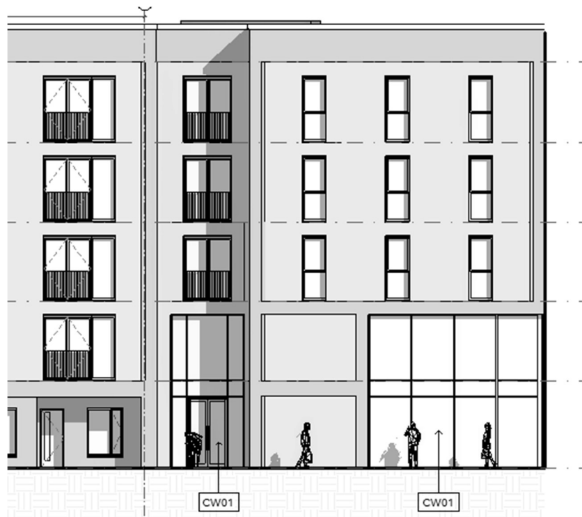
Figure 11.10.3.3 Elevation changes to windows from Level 2 to Level 4 Flat 002 Bedroom 01, Block B north façade
