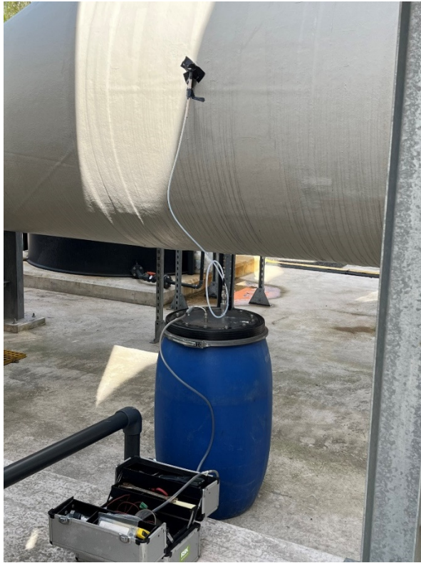
Figure 2.2: Odour Sampling Equipment Set-up – Location B
