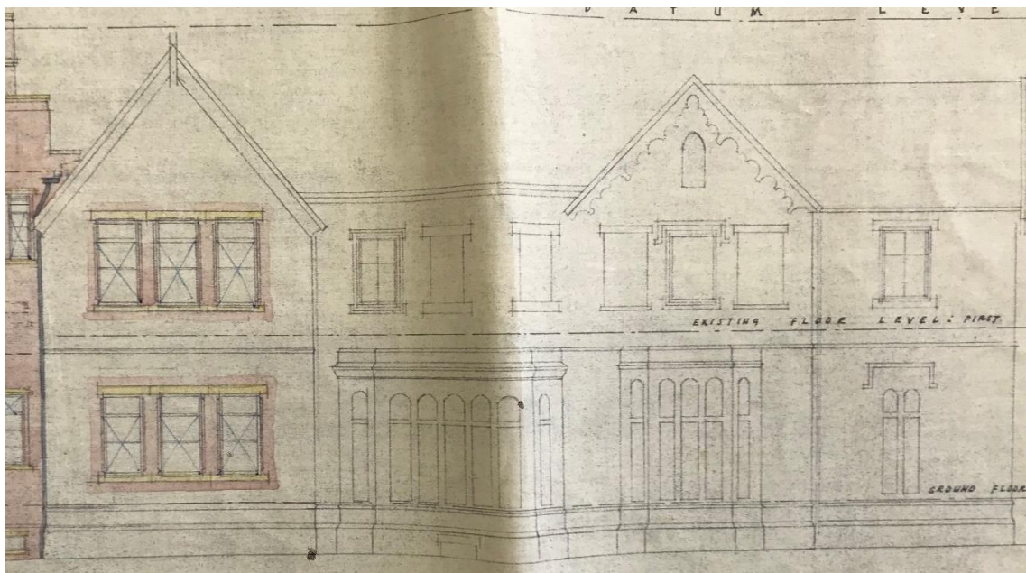
Figure 41 – The same view as detailed in the 1937 plans, showing the proposed alteration of the original first floor windows to the left, and the already altered first floor windows to the centre and right. Note the original Gothic stone mullioned windows to the centre and right of the ground floor are still present at this time.
