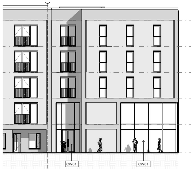
Figure 7.3.3.3 Elevation changes to windows from Level 2 to Level 4 Flat 002 Bedroom 01, Block B north façade
