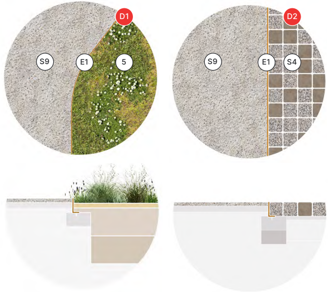
Interface between hard and soft landscape Interface between tarmac and reclaimed cobble
