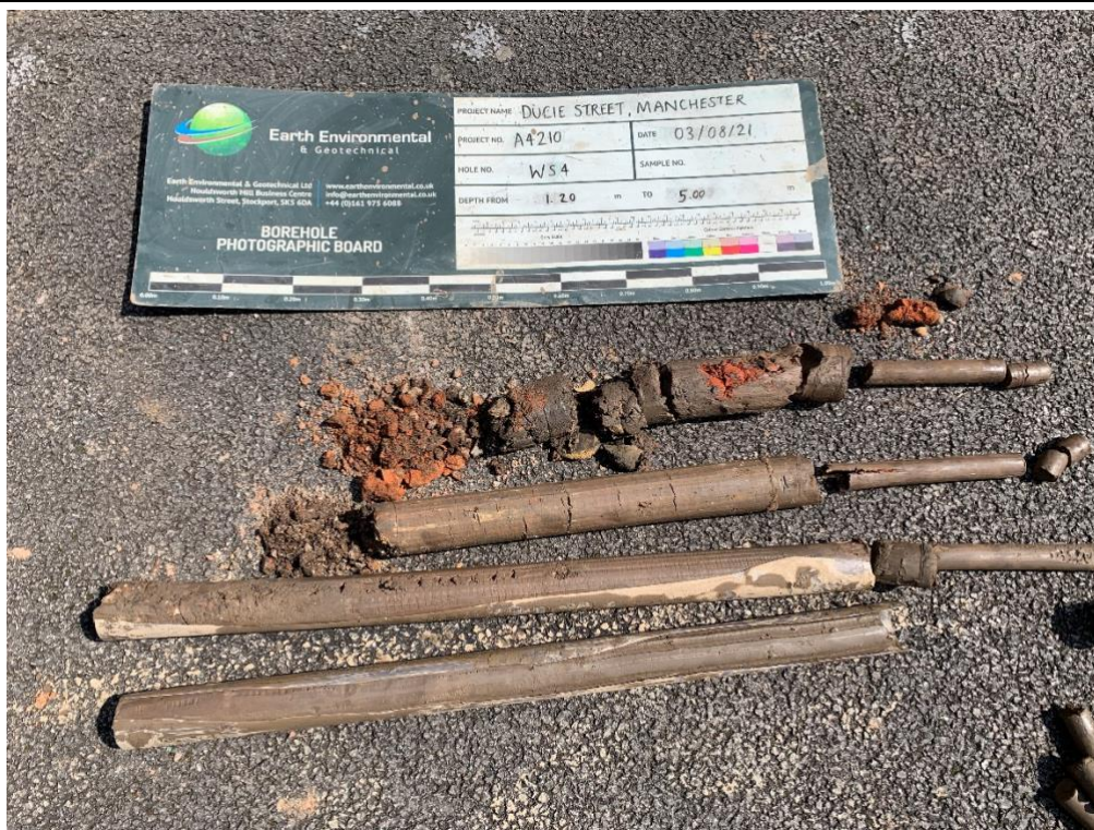
Figure 5 Made Ground and Superficial Deposits Encountered in the Window Sample Boreholes
