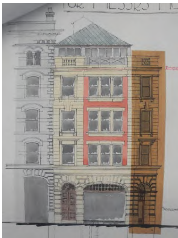
Figure 24: Elevation to High Street - August 1915, later altered to include ashlar stone to the upper floors instead of red brick.
