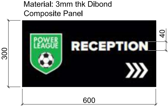
Location 6 Sign B (internally illuminated) Scale 1:10 @ A3
