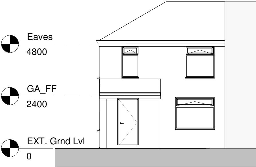
Existing Elevation North 1 : 100
