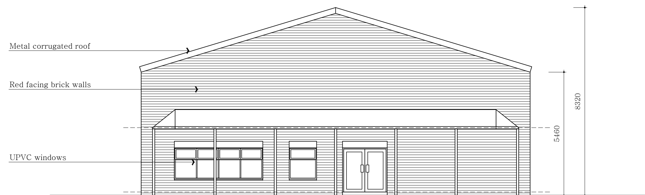
EXISTING FRONT ELEVATION (S) 1:100
