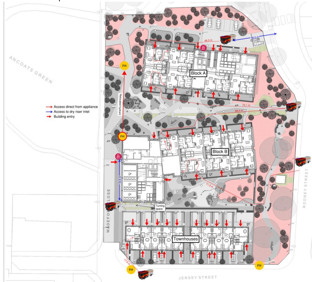
Figure 2 – FRS access to Site
