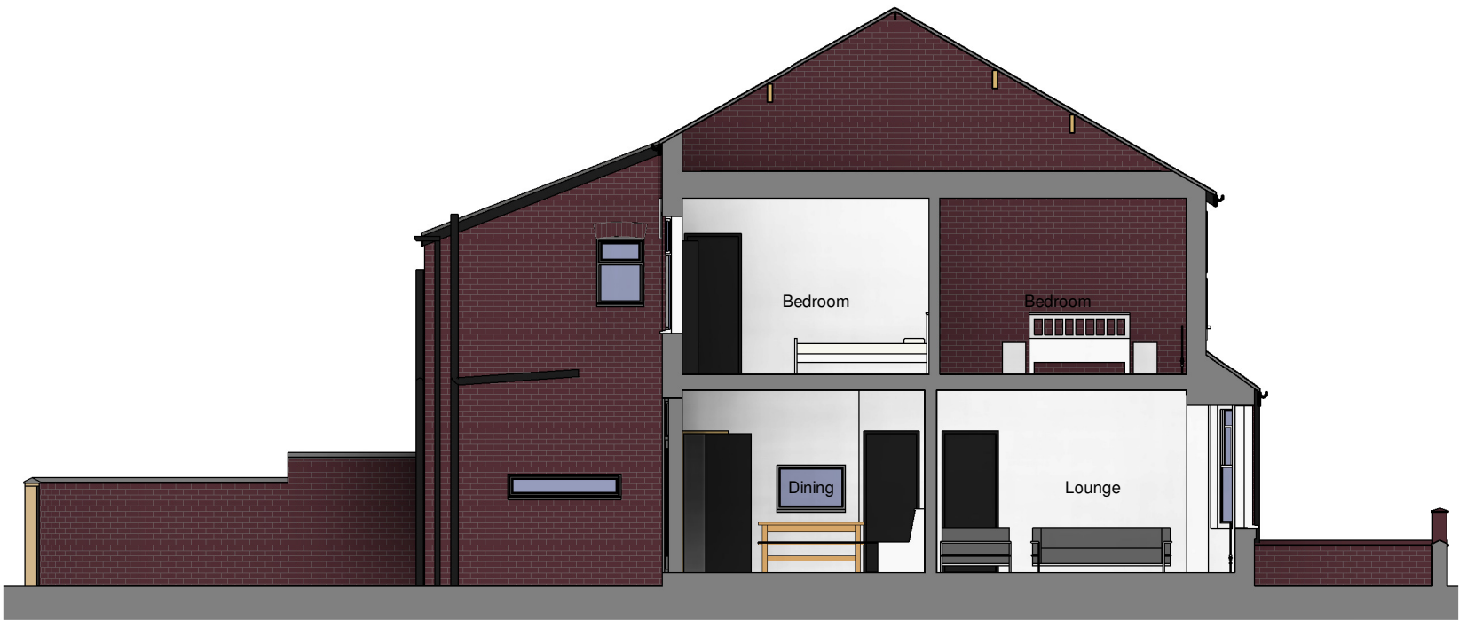
South West Elevation (Side) - Existing 1 : 100
