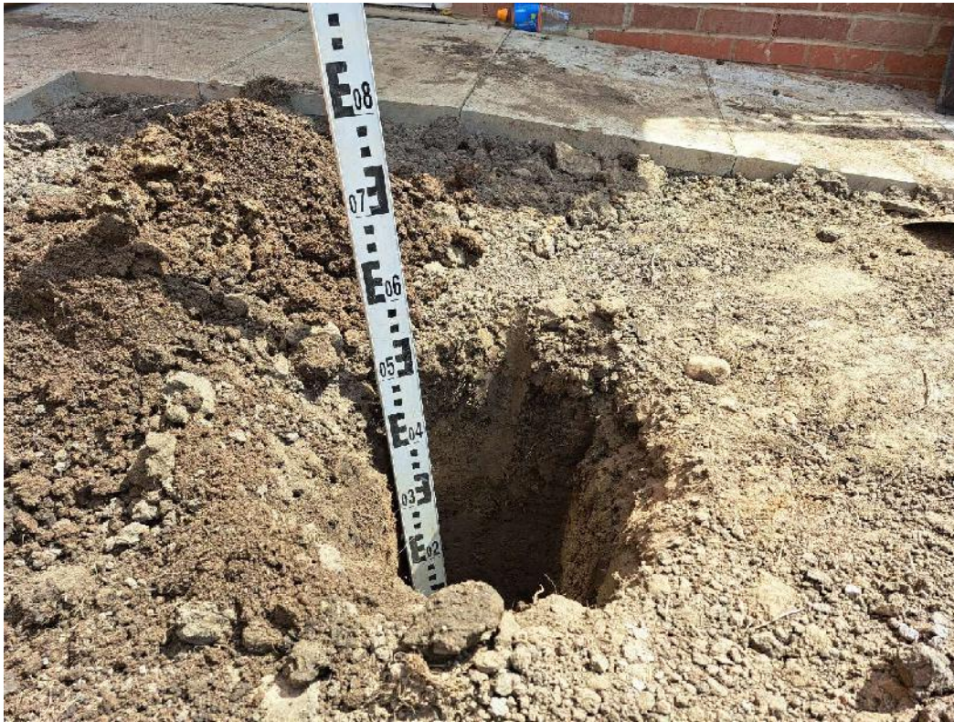
Photograph 11 350mm of subsoil exposed in VP04.
