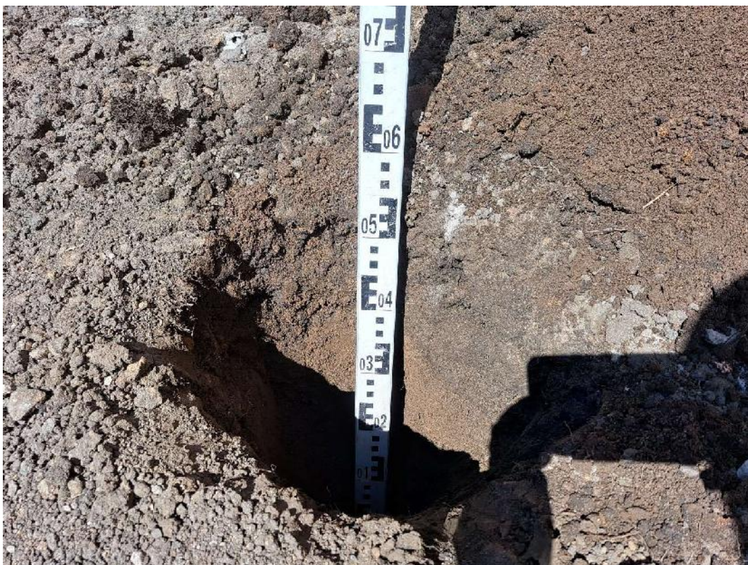
Photograph 8 300mm of subsoil emplaced in VP03.
