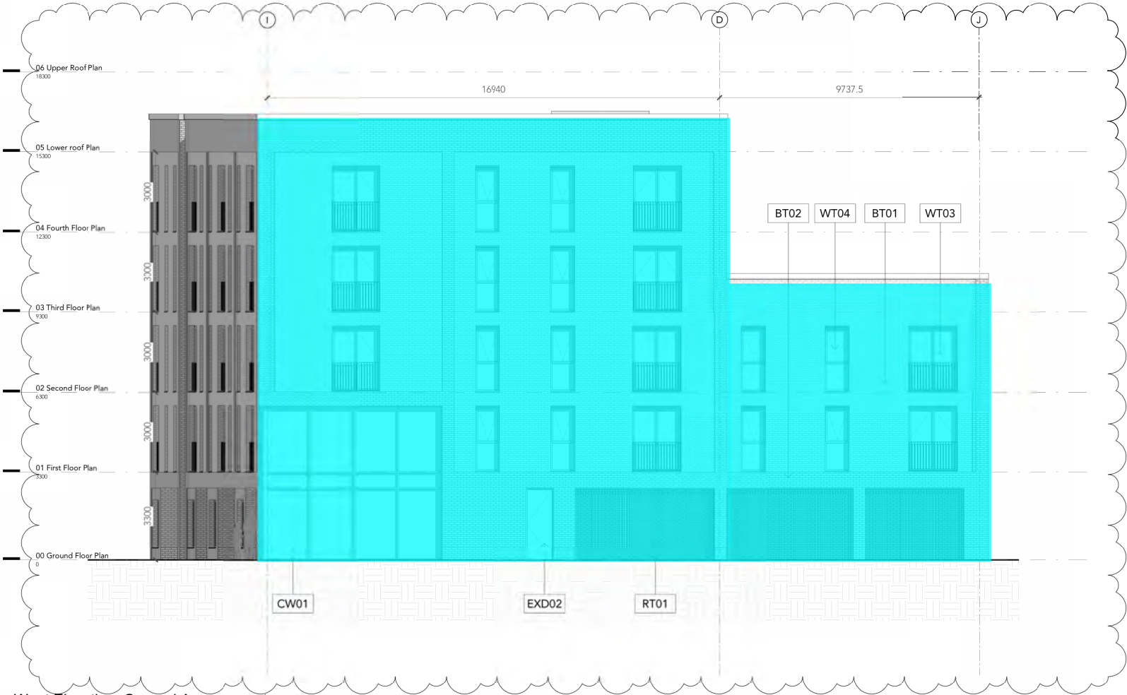
West Elevation_General Arrangement 1 : 100
