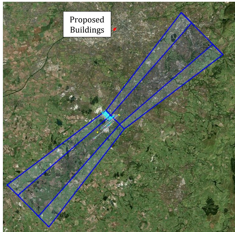
Figure 38. VOR/DME RWY 23R Protection Area
