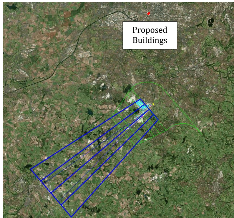
Figure 27. VOR/DME RWY 05R Protection Area
