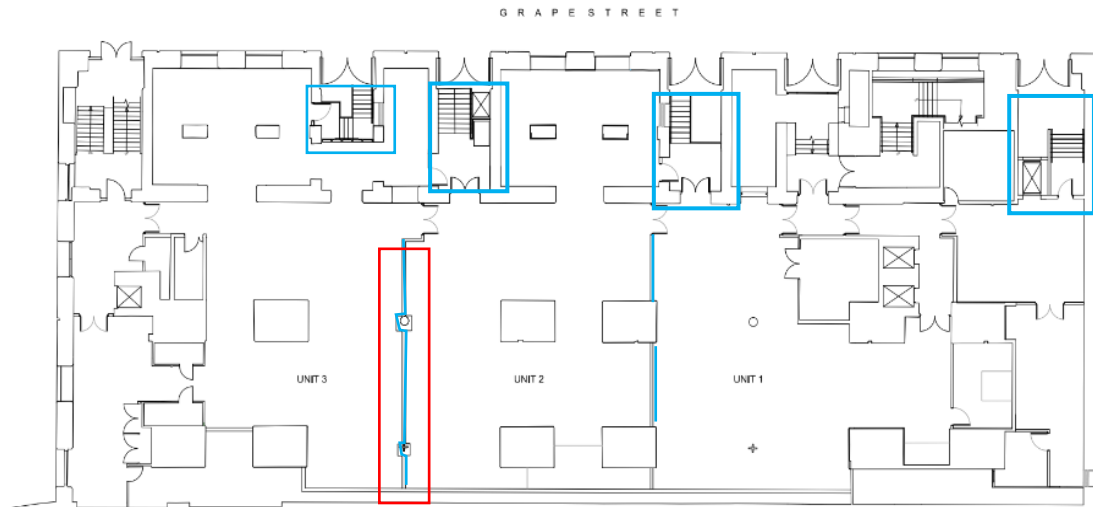
Figure 7: The Bonded Warehouse early 2018. Level 2 floor plan. The principal changes to the space (indicated in blue) include; stairs and service lifts to the north side and removal of former partitions / insertion of new partitions.
