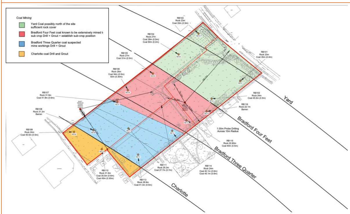
FIGURE 5.0 – AREA OF GROUTING REQUIRED
