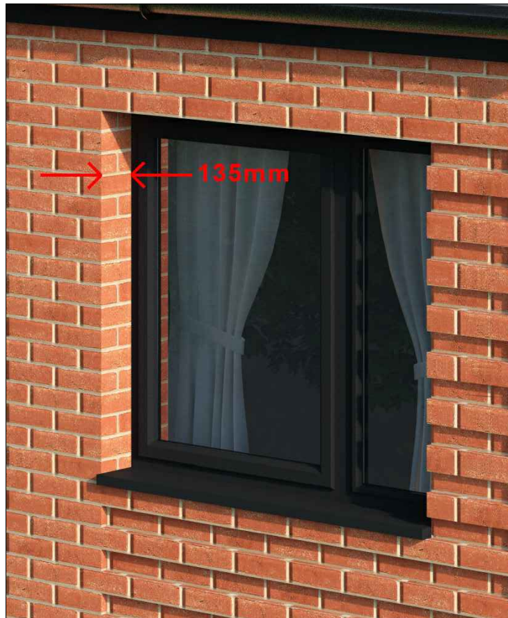
CGI image of proposed 135mm window reveal Not to schedule
