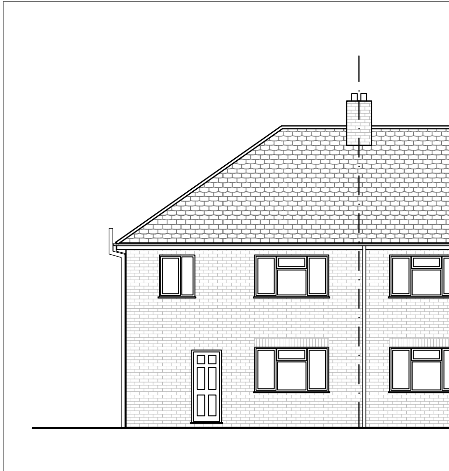
Rear Elevation as Existing Scale - 1:100
