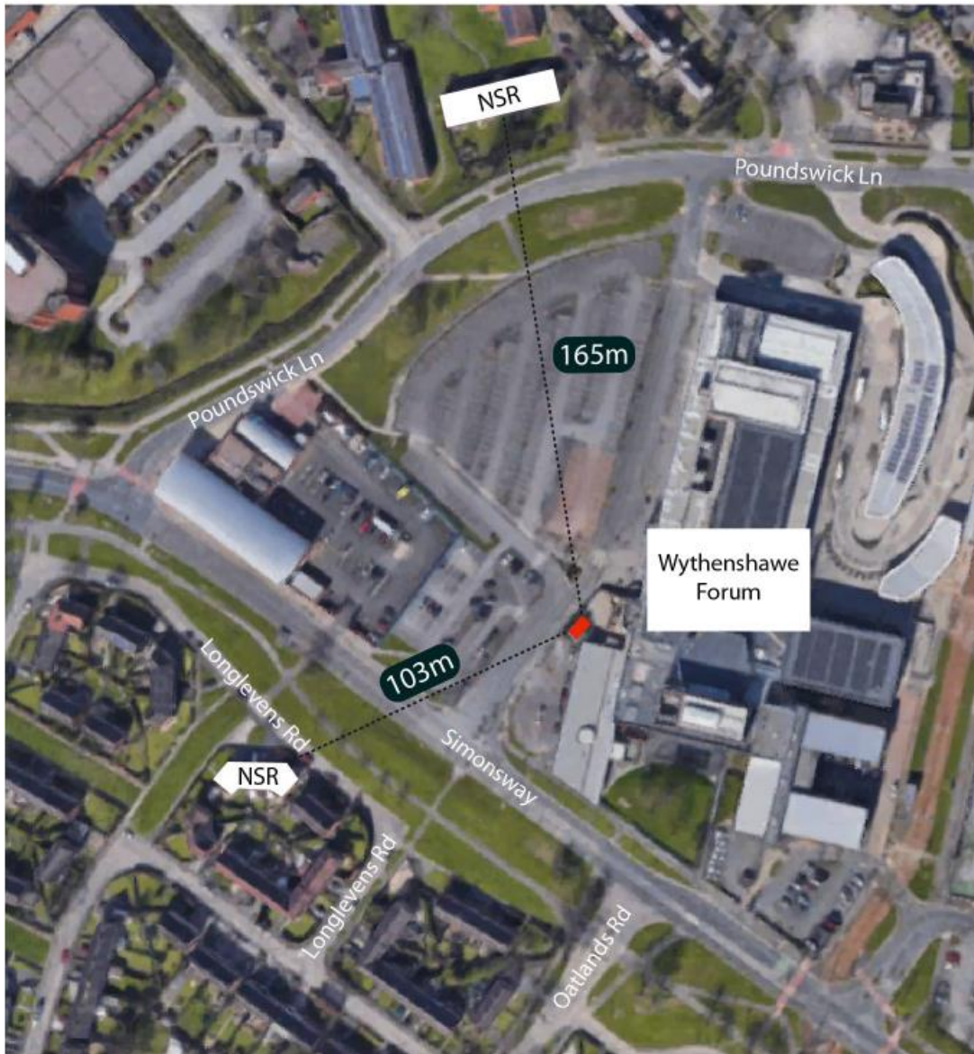
Figure 1: Location of installed plant highlighted in red and closest NSR properties highlighted in white
